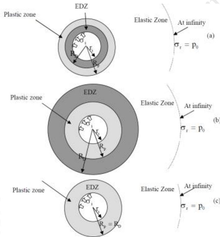
**Figure 1. The circular deep tunnel with a cylindrical EDZ: (a)  $R_p > R_D$  (b)  $R_p < R_D$  (c)  $R_p = R_D$**
