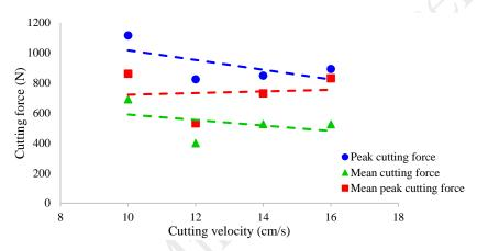
Fig. 2 Variation in cutting force with cutting velocity
