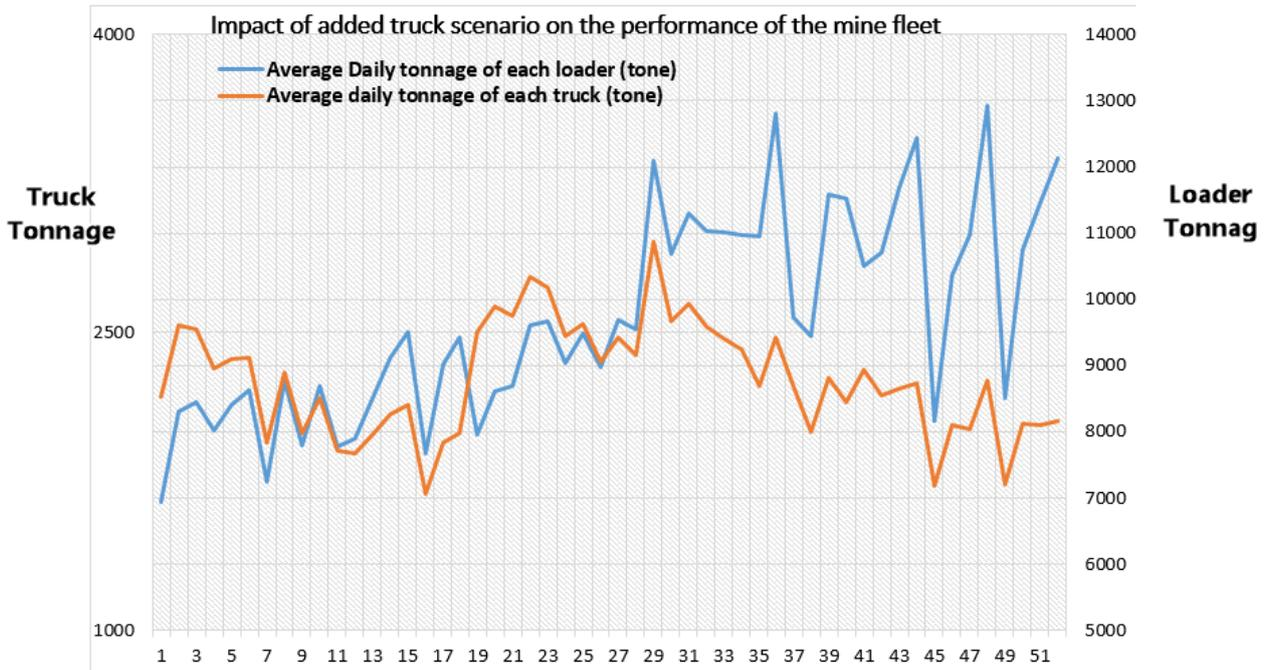
Fig 4: Comparison of changes in average daily tonnage of loader and truck for each of the scenarios on increasing the number of trucks
