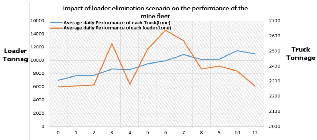
**Fig 3: Comparison of changes in average daily tonnage of loader and truck for each of the scenarios**
