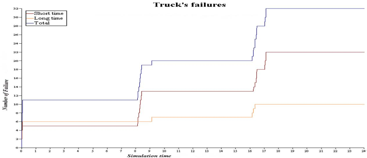
Figure 2: Simulation of the number of machine failures (short-term and long-term)
