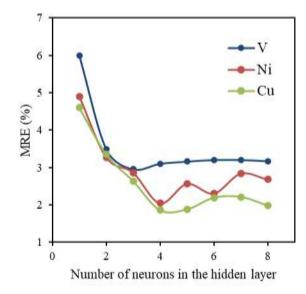
Figure 1. Relative error changes according to the number of neurons in the hidden layer.
