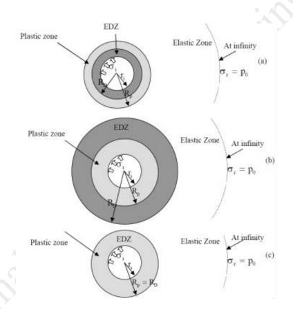
Figure 1. The circular deep tunnel with a cylindrical EDZ: (a)  $R_p > R_D$  (b)  $R_p < R_D$  (c)  $R_p = R_D$
