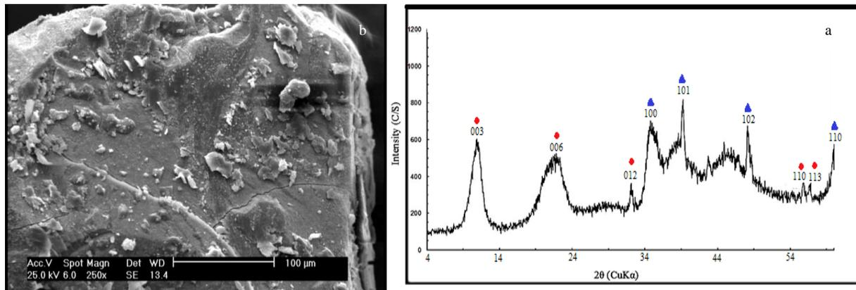
Figure 1. XRD spectra (a) and SEM image (b) of LDH
