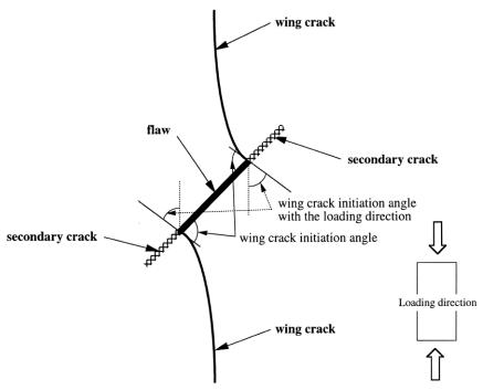
Figure 1. Schematic view of crack pattern in pre-cracked specimens of rock materials in uniaxial quasi-static compression (Bobet and Einstein 1998)
