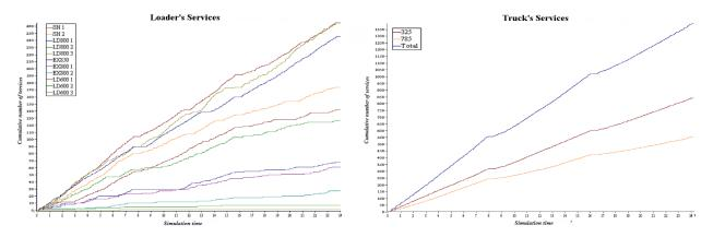
Fig.1: Simulation model output for the cumulative number of services by types of loaders and trucks
