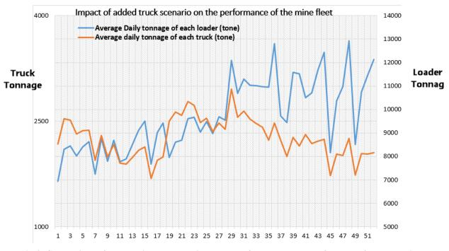
Fig 4: Comparison of changes in average daily tonnage of loader and truck for each of the scenarios on increasing the number of trucks
