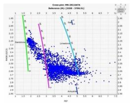
Fig. 2. Log of density versus photoelectric
