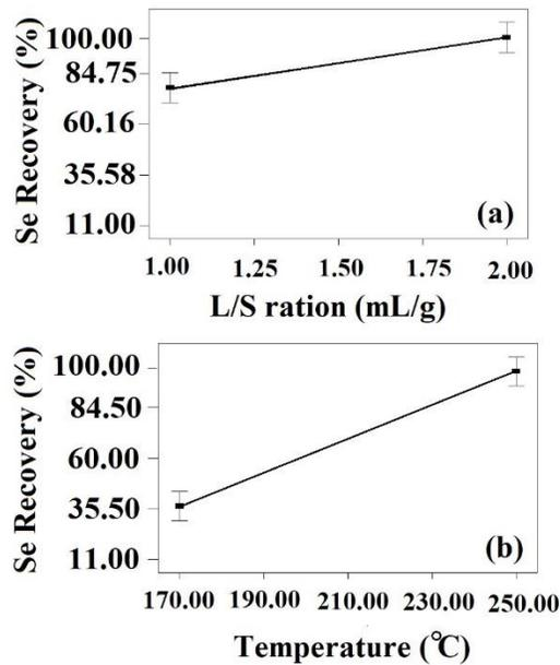
**Figure 1. The effect of the L/S ratio (a) and the temperature (b) on the recovery of selenium.**
