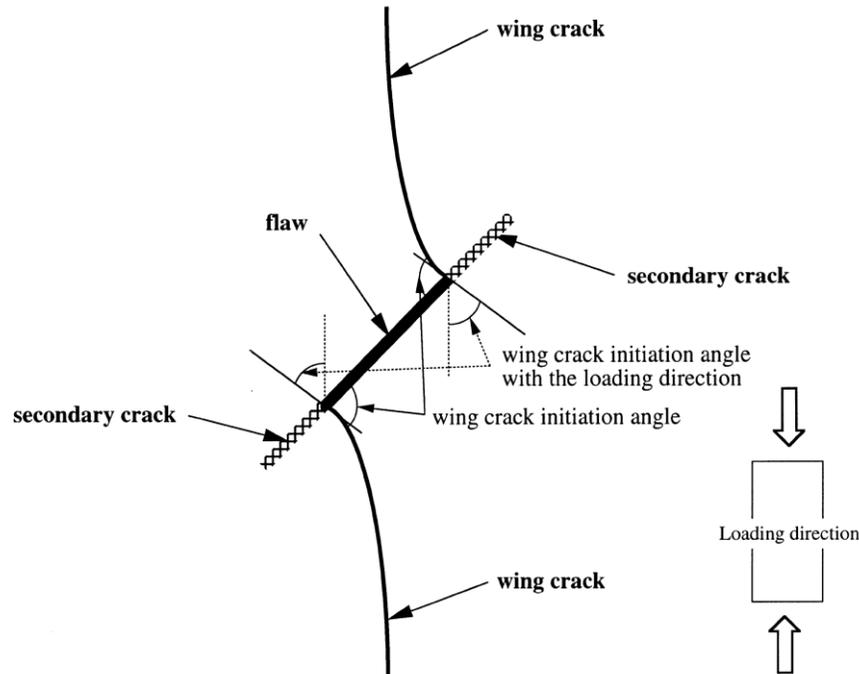
**Figure 1. Schematic view of crack pattern in pre-cracked specimens of rock materials in uniaxial quasi-static compression (Bobet and Einstein 1998)**
