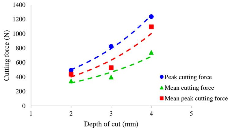
Fig. 1 Variation in cutting force with depth of cut
