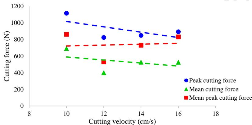
Fig. 2 Variation in cutting force with cutting velocity
